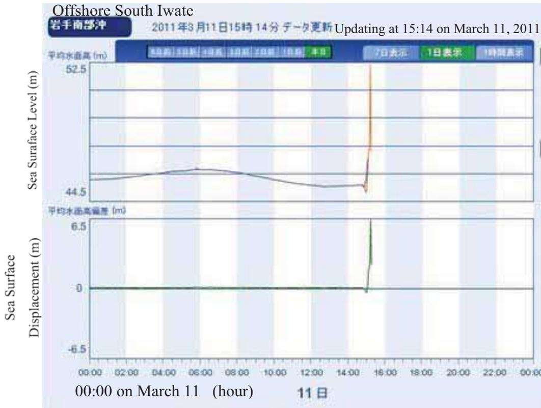
**Figure 13.** Tsunami due to Tohoku-Oki earthquake on 11th March 2011 by a GPS buoy. Real time 24hr data of GPS buoy at Off South Iwate (Kamaishi) (<http://www.mlit.go.jp/kowan/nowphas/>)
