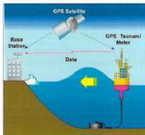
Fig. 1. Concept of GNSS buoy for tsunami early warning [1].
