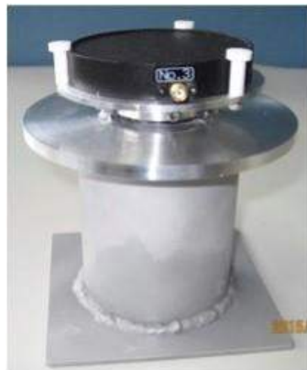
Picture 2: The antenna set on the manufactured gimbal apparatus.
