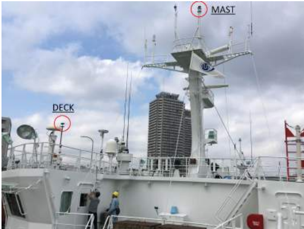
Fig. 1 GNSS antennas installed on the top deck (DECK) and on the mast (MAST) of the RYOFU MARU on October 19, 2017. The MAST antenna was moved to the DECK location on June 19, 2017, and was used for additional observations as DECK until August 6, 2017
