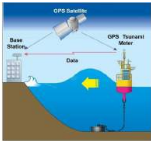
Fig. 1: Concept of GNSS buoy for tsunami early warning.
