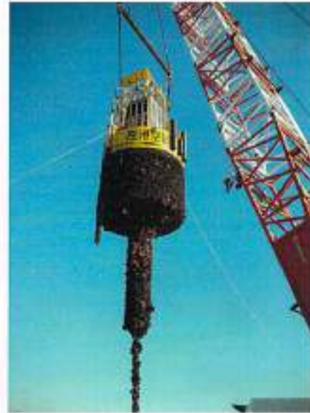
Fig. 2. Buoy after three years and seven months of operation off Cape Muroto, Japan [9].
