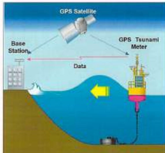
Fig. 1. [Coke online] Principle of GNSS buoy for measuring tsunamis. [1]
