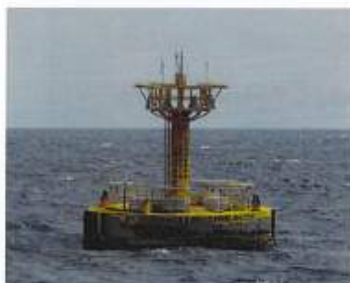
Fig. 5. Fishery buoy No.18, operated by Kochi Prefecture and used for the present study. On the top of the center pillar is the GNSS antenna. On the deck of the buoy are solar panels and other apparatuses.
